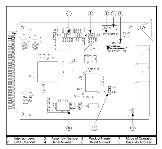
Figure 2-3 shows the location of the configuration jumpers and switches on the STD-GPIB.
